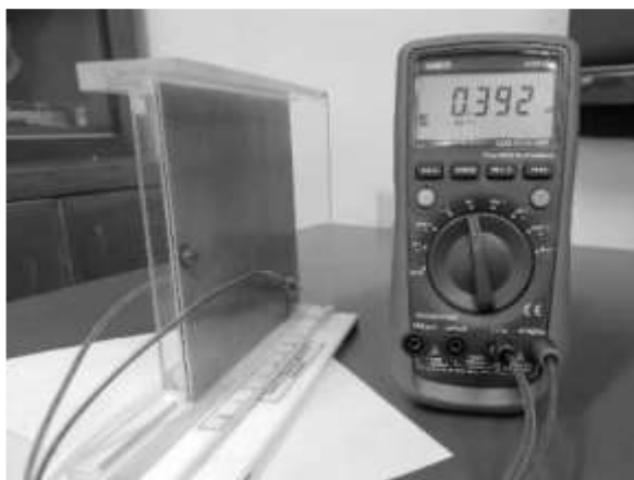
Figure 3. The digital capacitance meter (right) showing the initial capacitance of an air parallel-plate capacitor at 0.392 nanofarad
