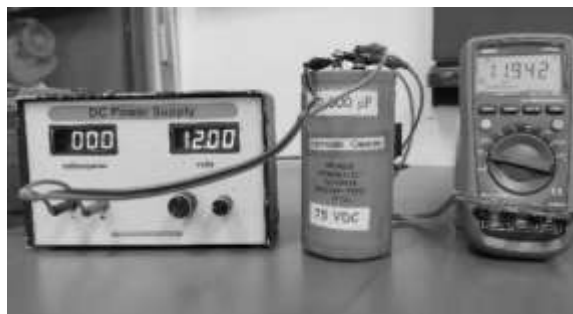
Figure 5. This part of the demonstration shows that charging a capacitor ends when the capacitor voltage (shown in the digital multimeter at 11.942V) and voltage source (shown in the built-in voltmeter of the DC power supply at 12.00V) are equal.
