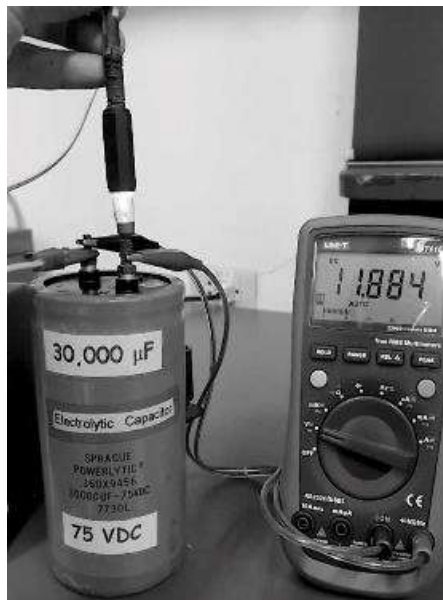
Figure 6. A bulb is shown at the onset of discharging the 30,000-microfarad electrolytic capacitor (digital multimeter showing the initial capacitor voltage at 11.884V).
