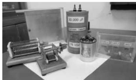
Figure 1. A set of various capacitors (from L-R: variable air capacitors, electrolytic capacitors, and ceramic capacitors of varied sizes and capacitances)
