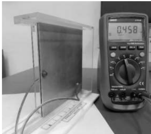
Figure 4. The digital capacitance meter (right) showing the increased capacitance of an air parallel-plate capacitor at 0.458 nanofarad
